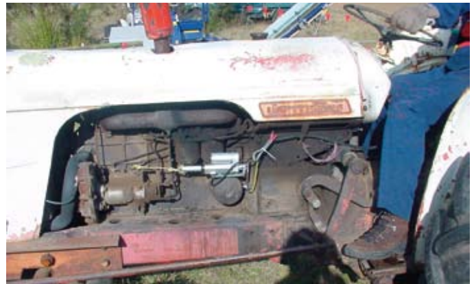
Aged David Brown tractor with radio control throttle attached
